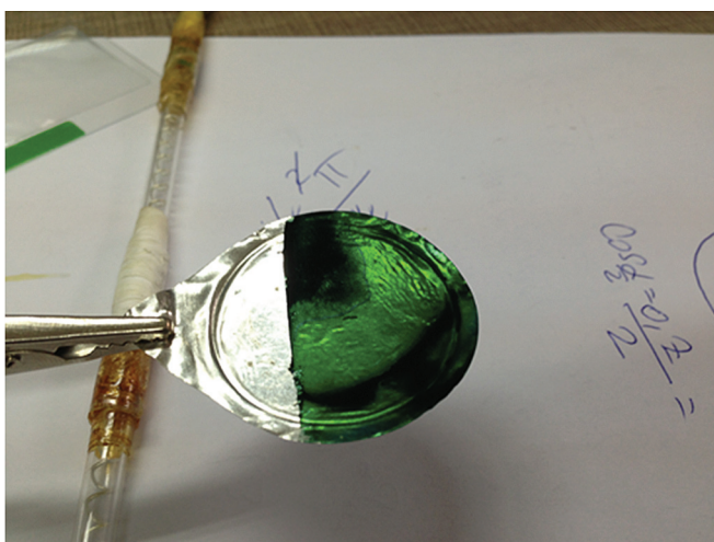
Fig. 3. a) Dark blue deposit of oxidized PANI b) green deposit of electroconductive PANI. (For interpretation of the references to colour in this figure legend, the reader is referred to the web version of this article.)
