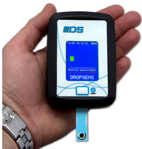
Fig. 3 Portable hand-held electrochemical instrument to obtain the heavy metal levels
