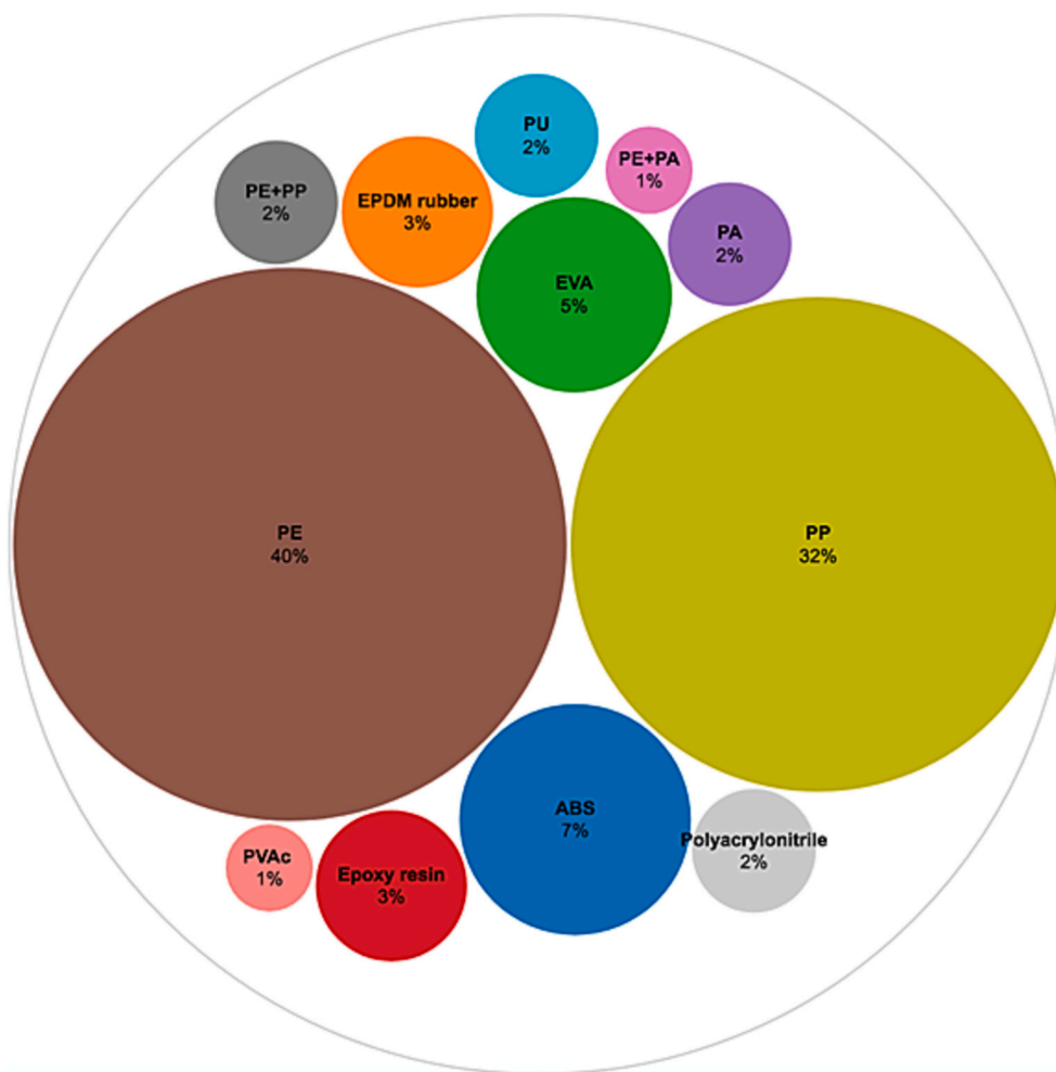
Fig. 4. Circle packing chart of the proportions of the different polymers identified in the particles collected from Brazilian coastal beaches by ATR-FTIR spectroscopy. ABS = Acrylonitrile Butadiene Styrene; EPDM = Ethylene Propylene Diene Monomer rubber; EVA = Ethylene Vinyl Acetate; PA = Polyamide; PE = Polyethylene; PP = Polypropylene; PU = Polyurethane; PVAc = Polyvinyl Acetate; PE + PP = Polyethylene and Polypropylene blend; PE + PA = Polyethylene and Polyamide blend.
