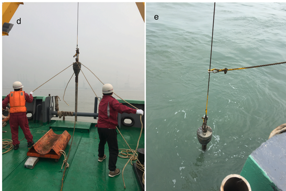
Fig. 1. Sampling locations for sediment cores, and the historical change of coastline and coastal land reclamations during 1970–1984 and 1984–2017 in Xiamen Bay (a–c) (Lu et al., 2011). The surface sediment migration trend was modified from (Cai et al., 1999; Fang et al., 2010b; Zuo et al., 2011). Sediment core sampling in Xiamen Bay, China (d,e).
