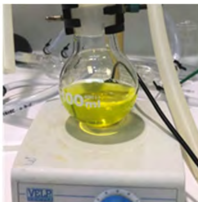
Figure 25. reaction set-up for the fluorescent labelling of PLA nanoparticles.
