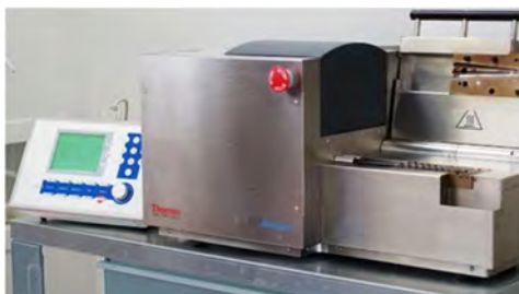
Figure 1. Laboratory extruder HAAKE™ MiniLab II Micro Compounder.
