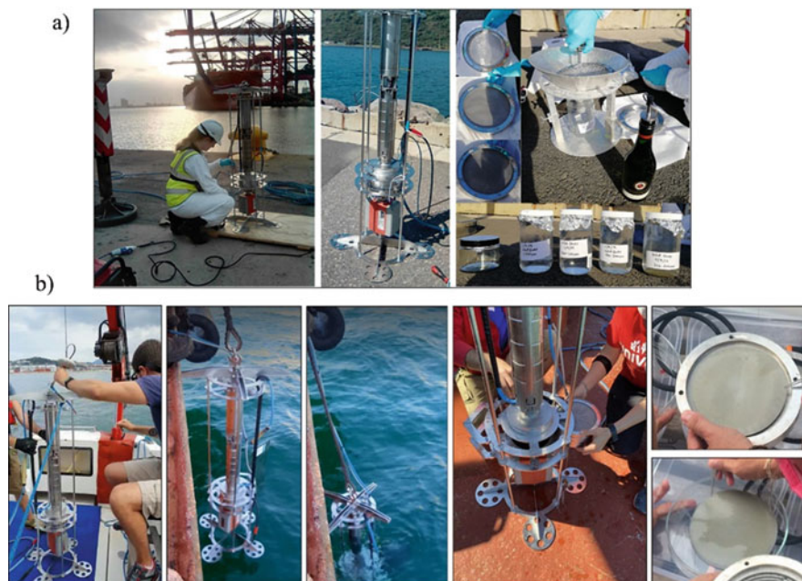
Fig. 8.4 Micro Plastic Particle Pump (KC Denmark) as an example of submersible device for sampling microplastics in seawater. (a) Operation of the pump in a port environment and sample collection (modified from Preston-Whyte et al. 2021). (b) Operation of the pump and sample collection carried out by the Polytechnic University of Marche (Italy) along the coasts of Adriatic Sea during activities of RESPONSE project funded by JPI Oceans, 2020–2023 (photo credit, S. Gorbi and F. Regoli)
