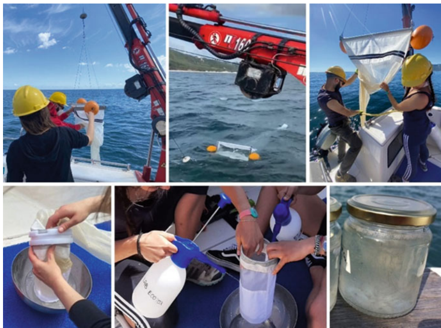
Fig. 8.2 Net-based method for sampling microplastics in surface waters. Activities carried out by the Polytechnic University of Marche (Italy) in the Adriatic Sea using a manta net during activities of RESPONSE project funded by JPI Oceans, 2020–2023 (photo credit, L. Pittura and C. Mazzoli)
