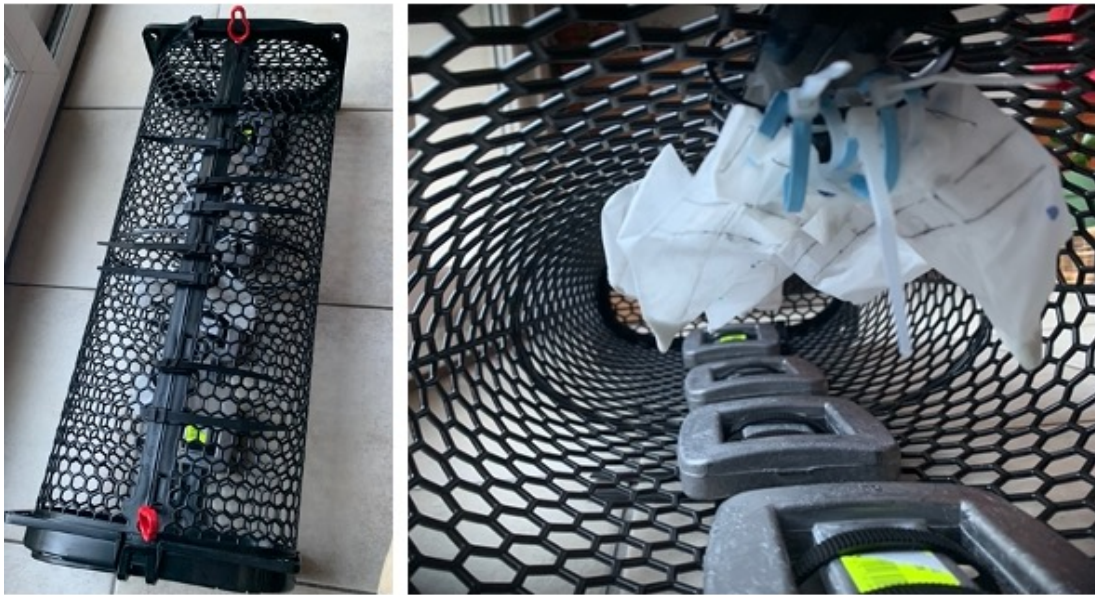
Image on the left: Incubation device ready to be installed on in the sea. Image on the right: A photo showing the inside of the incubation device.
