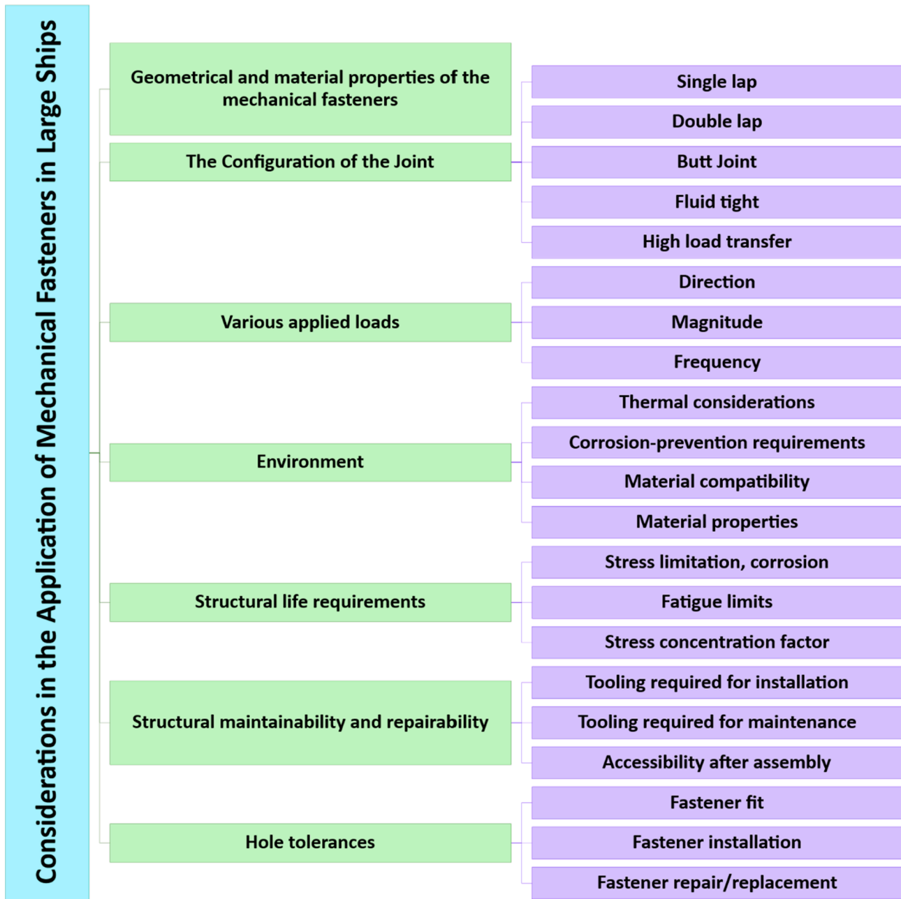
Fig. 28. Consideration regarding the application of the mechanical fasteners in the large ships.
